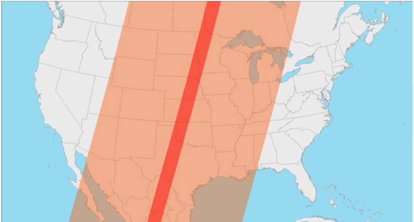
Figure 1 - Example of a 185 km Landsat 9 OLI swath (red) compared to a 2,330 km Terra MODIS swath (orange). Terra MODIS can easily image the entire continental US daily in three consecutive orbits. However, Landsat 8 and Landsat 9 OLI each require multiple orbits over 16 days to provide the same coverage.
