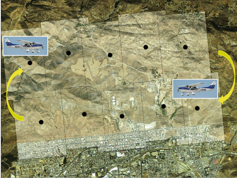
Fig. 5 Illustration of repeat pass, high temporal resolution imaging using a racetrack pattern. The location is Tecate, CA along the U.S./Mexico border
