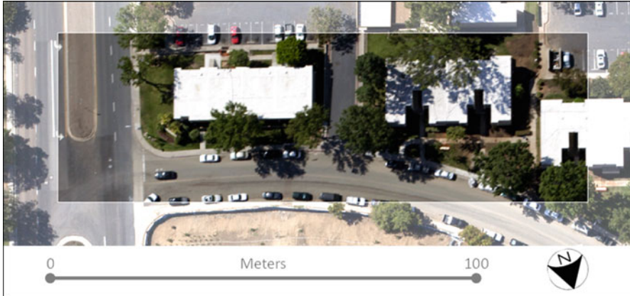
Fig. 2 A time-2 image chip is overlain on a time-1 image displayed in a lighter tone (i.e., washed-out). The quality of the spatial co-registration between the 8 cm (3 in) spatial resolution image sets is evident, as linear features such as street curbs, parking space paint lines, and roof edges are precisely aligned. A vehicle turning the corner is only present in the smaller image chip (half of the vehicle), while that vehicle was not present during collection of the larger image chip
